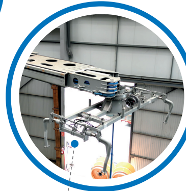
FRIGATE (SPANISH NAVY) MULTIMISSION BAY HANDLING SYSTEM
