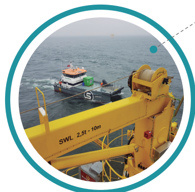
JACKET CRANE MAN RIDING CAPABILITY AND CONSTANT TENSION
