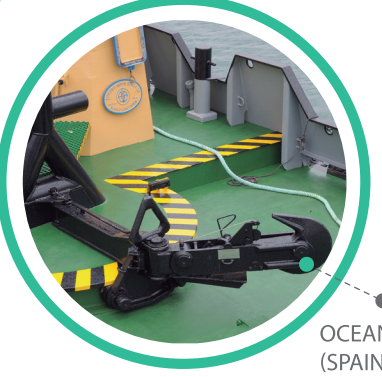
OCEAN-GOING TUGS (SPAIN) 400T TOW PIN WITH 500T FORK
