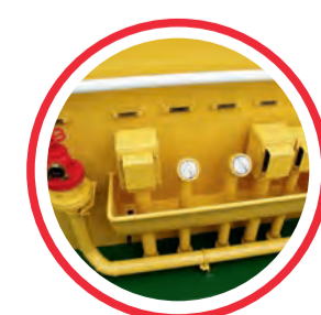
TANK VENT VALVES
